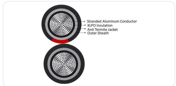
Figure 1 — Cross section of both cores: stranded aluminium conductor, cross linked insulation, anti termite jacket, outer sheath.
