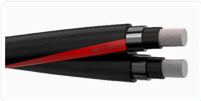
Figure 2 — Two single cores twisted, cut back to the stranded aluminium conductors. Core identification black and black with red strip.
