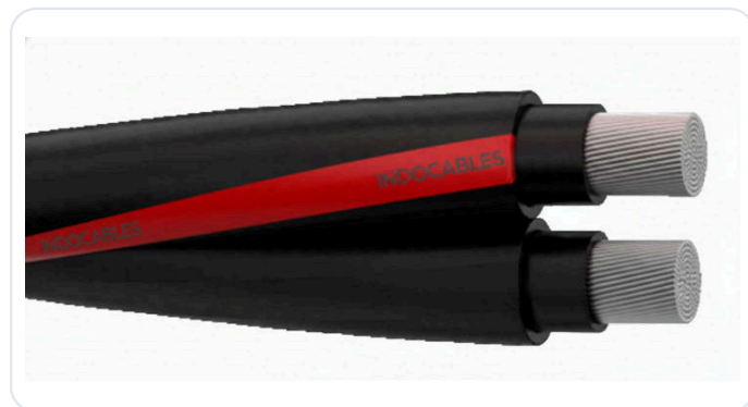
Figure 1 — Two single cores twisted, cut back to the stranded aluminium conductors. Core identification black and black with red strip.
