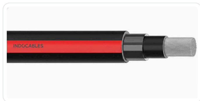
Figure 2 — Single core cable stripped back through sheath, nylon jacket and insulation. Core identification black and black with red strip.
